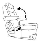
Ensure seat is latched to vehicle floor by pushing/pulling on seat. If not latched, the seat may cause injury during a sudden stop.
